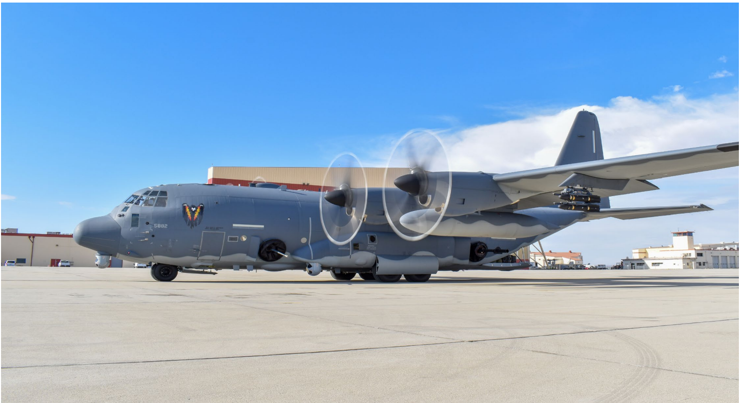
The AC-130J is a highly modified C-130J aircraft that contains many advanced features, such as an advanced two-pilot flight station with fully integrated digital avionics. (Photo Credit: U.S. Air Force)
