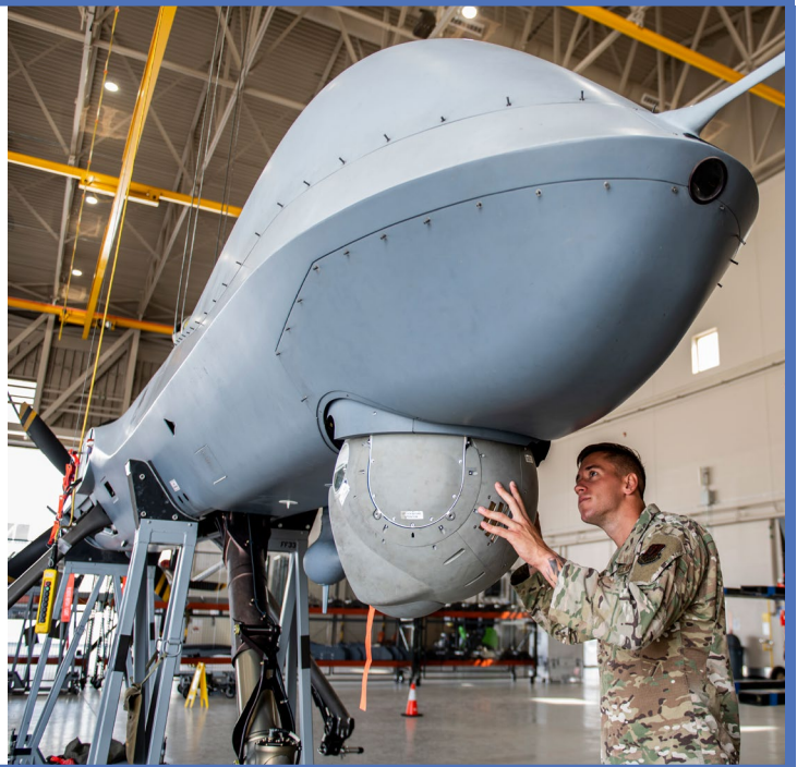
Senior Airman Levi, 432nd Aircraft Maintenance Squadron crew chief, checks out the multi-spectral targeting system on an MQ-9 Reaper at Creech Air Force Base, Nevada. (Photo credit: Senior Airman William Rio Rosado)
